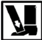
The module drawers, shelves and their contents are heavy and could cause injury if they fall onto or strike personnel. A tilt hazard exists when the module drawer is extended, but not locked down to the base plate. As a rule, always work on one drawer at a time. Never have more than one drawer extended in the full open position at a time, especially if loaded with material. Personnel should never stand on a drawer.
