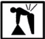
The module drawers and shelves can be heavy and awkward to handle by a single person. This is especially true of the larger components. The movement of these items is a two-person operation for empty drawers. Assistance is required from one or more personnel to separate and remove drawers from the frame of each assembly. DO NOT remove or lift QUADCON module drawers without assistance; injury to personnel will occur.
