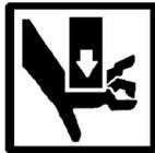
Standard forklift principles apply when working on the QUADCON Modules. When working with ground guides during the loading or unloading of a module, never move the QUADCON Modules into the container while the ground guide is between the fork, QUADCON Modules, and the container. Serious injury could occur if the ground guide is pinned between the forklift and the container. Forklift operators must maintain visual contact with their ground guides at all time.
