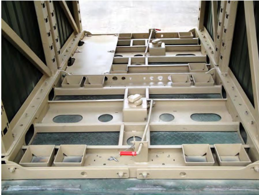
28. Return to the Floor Adapter connection bolts; tighten both left and right bolts and nuts.
