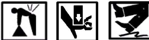
Use proper lifting techniques when lifting the QUADCON Adapter. Use work gloves when handling the Adapter. Never use fingers to align the bolt holes. Ensure that there is proper footing when moving lifting or positioning the Adapter.
