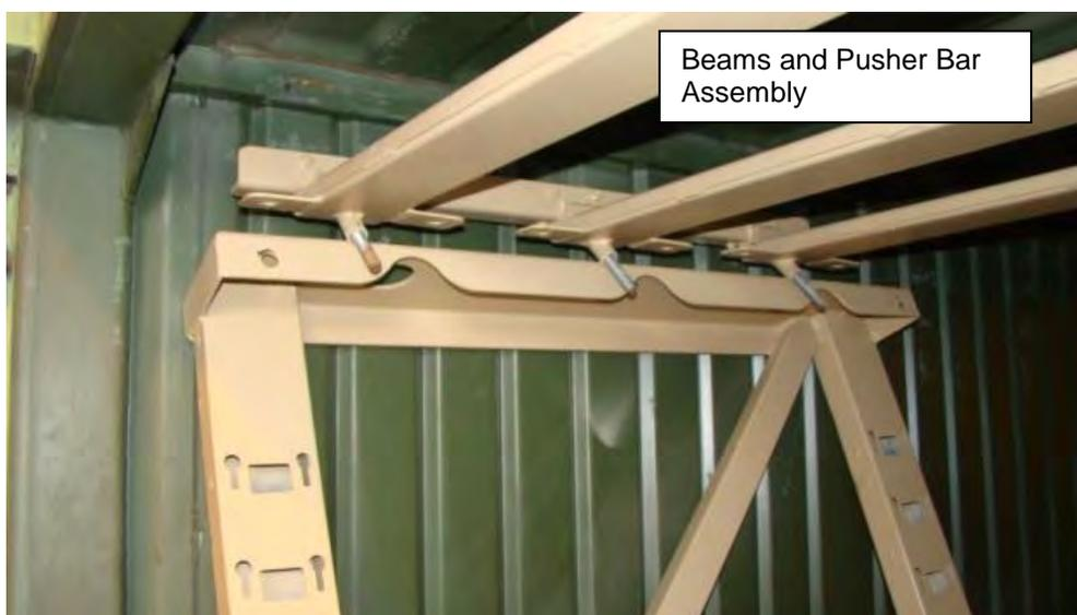
11. With assistance, place each adjustment bolt through the openings in the top of the frame as shown on both sides.
