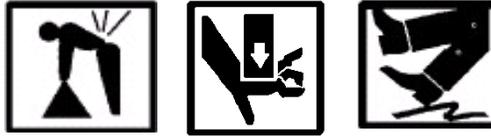
Assistance is required for the following assembly steps. Use proper lifting techniques when lifting the frames and assembled beams. Use work gloves when handling all restraint parts. Never use fingers to align the bolt holes. Ensure that there is proper footing when moving, lifting or positioning the frames.
