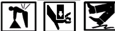
Use proper lifting techniques when lifting the QUADCON Adapter. Use work gloves when handling the Adapter. Never use fingers to align the bolt holes. Ensure that there is proper footing when moving, lifting or positioning the Adapters.
