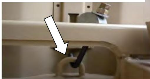
1. When installing the J hook bolts, select a hole near the tie down ring, then angle the J-bolt about 20 to 30 degrees toward the center.
