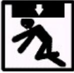
Do not allow the Light Expeditionary Module (LEM) system to swing if using an overhead lift. Always ensure an appropriate sling and lifting points are used in lifting the LEM. Always use properly sized forklift, crane, or lifting device. Failure to comply could cause injury, death or damage to the equipment.
