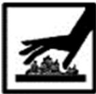
Protective gloves should be worn when handling metal parts in high temperatures. Failure to wear gloves may result in burning or blistering of the skin upon contact.
