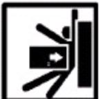
A tilt hazard exists when forklift operators try to lift the LEM module without the forklift tines fully inserted in the fork pockets provided in the base. A tilt situation exists when the heaviest part of the load is out on the tips of the tines or on uneven ground while traveling. Operators should always keep loads low and close to the forklift carriage. Operators should never travel when the load is in the fork's extended position.
