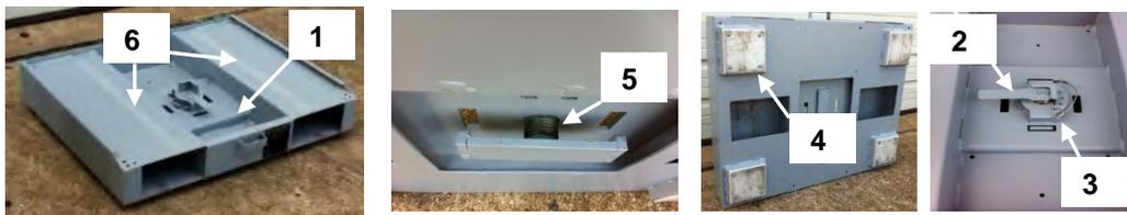
1. Inspect the cabinet base (1) for dents, weld cracks or damage, report damage to maintenance.
