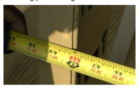
8. Install the *third* vertical rack following steps 3 through 5 above. Measure **30-inch** from the inside of the second rack to the inside of the third rack. Once the correct measurement is verified at all four points on the vertical rack frame, tighten the bolts on the top and bottom mounting plates using a ¾-inch socket and ratchet.
