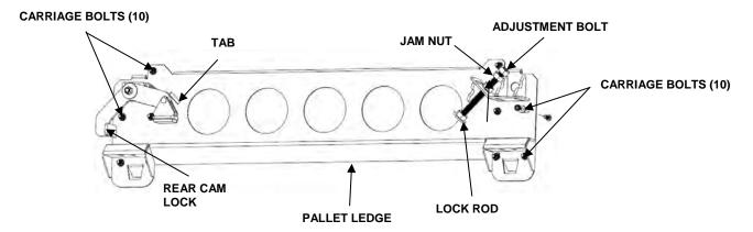
15. Pallet ledges are retained on the vertical rack frame by ten ¼-inch carriage bolts and four bayonet tabs protruding into the windows of the vertical rack frame. This requires the ledge to be loosened from the vertical rack frame. While one person securely holds the pallet ledge, the second person applies an upward force by tapping the underside of the ledge at the attached point with a 2 X 4 soft wooden block or similar material.
