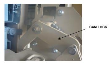
29. Tighten jam nut using 7/8-inch combination wrench to hold lock rod in the closed position.
