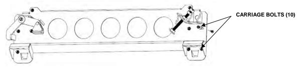
11. Place the pallet ledges in their desired positions by inserting the bayonet tabs into the vertical rack frame windows while aligning the ten carriage bolts into their appropriate slots.
