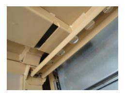
17. Install rear pallet ledge stabilizer with four Button Head Bolts with 5/16-inch lock washers using 3/16-inch hex driver socket and 3/8-inch ratchet with extension from the two positions of each pallet ledge. There are four bolts located at each vertical rack frame.
