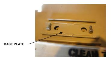
Install (4) unistrut channel nuts to each base plate and (2) unistrut channel nuts to the mounting channel in ceiling at approximately the locations described in steps 6 through 9 below.
