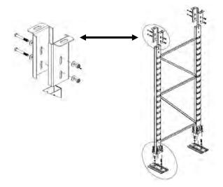
5. Secure upper sleeves to ceiling mount using (4) 1-inch bolts, (4) ½-inch lock washers, and (4) ½-inch flat washers. Apply Locktite 262 to bolt threads and hand tighten only.
