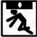
Forklift operator should always use module forklift pockets when moving FPU modules to prevent tipping. Ground guides must insure no personnel go underneath modules during movement operations. Failure to comply could cause injury, death or damage to the equipment.
