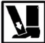
The Modules and their contents are heavy and could cause injury if they fall onto or strike personnel. A tilt hazard exists when the drawer is either not latched or frames have not been secured to the base plate. As a rule, always work on one drawer at a time. Never have more than one drawer extended in the full open position at a time, especially if loaded. Personnel should never stand on a drawer.
