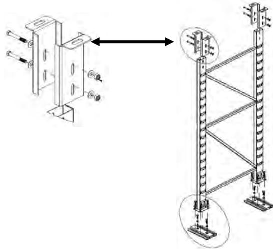
5. Secure upper sleeve to ceiling mount using (4) 1-inch bolts, (4) ½-inch lock washers, and (4) ½-inch flat washers. Apply Loctite 262 to bolt threads and hand tighten only.
