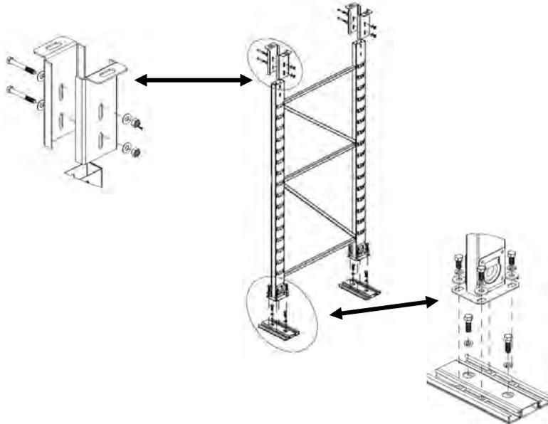
10. With someone holding the vertical rack frame, remove the 1/2-inch hex head bolts and washers from the top (2) and bottom (4) mounting plates using a 3/4-inch socket with ratchet.
