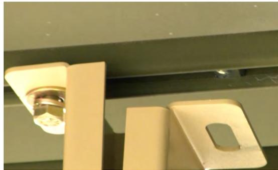
6. Install vertical rack frames from right to left beginning with the **first** vertical rack at the far right. Measure **8 1/8-inch** from the inside of the container frame to the outside of first vertical rack frame. Once the correct measurement is verified at all four points on the vertical rack frame, tighten the bolts on the top and bottom mounting plates using a ¾-inch socket and ratchet.
