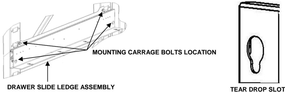
13. Apply Loctite 262 to the four ¼-inch nuts on the carriage bolts for each slide ledge.
