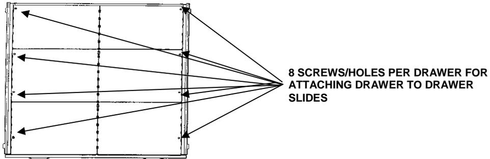
1. Fully extend drawer to the open position. (If drawer will not stay in the open position, this task will require two people. One to hold the drawer in the extended position and the other to perform drawer removal task).
