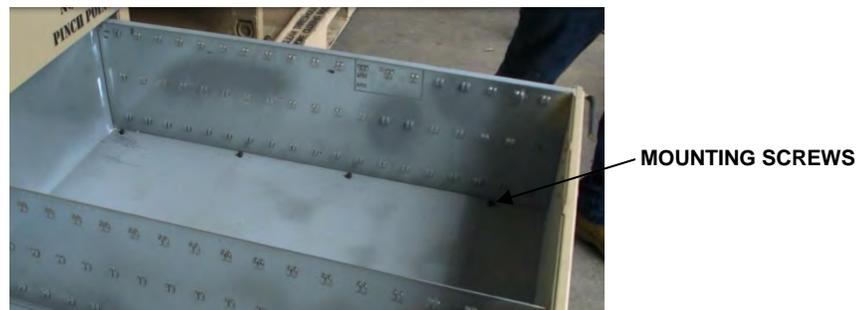
20. After hand tightening, push drawer completely closed and pull back to the full open position to allow drawer to seat into its proper location on the drawer slide ledge.
