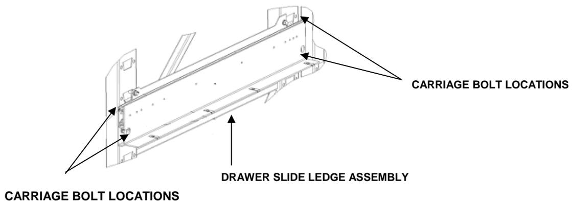
7. Slide ledges are retained on the vertical rack frame by four bayonet tabs protruding into the windows of the vertical rack frame. This requires the ledge to be loosened from the vertical rack frame. While one person securely holds the slide ledge, the second person applies an upward force by tapping the underside of the ledge at the attached point with a 2 X 4 soft wooden block or similar material.
