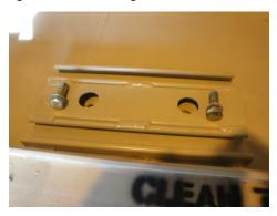
2. Install (4) unistrut nuts to each base plate and (2) unistrut nuts to each ceiling mount in the provided slots at approximately the locations described in steps 6 through 9 below.
