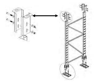
5. Secure upper sleeve to ceiling mount using (4) 1-inch bolts, (4) ½-inch lock washers, and (4) ½-inch flat washers. Apply Locktite 262 to bolt threads and hand tighten only.
