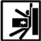
Use extreme caution when loading or unloading the FPU to or from a transport vehicle. Keep hands, fingers, and feet clear of the container and components during this operation. Forklift support is required. Make sure all container connectors are properly seated and locked secure. Failure to comply could cause serious injury or death or damage to the equipment.
