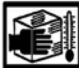
In extreme cold conditions, do not touch metal parts with bare hands. Severe skin damage may result.
