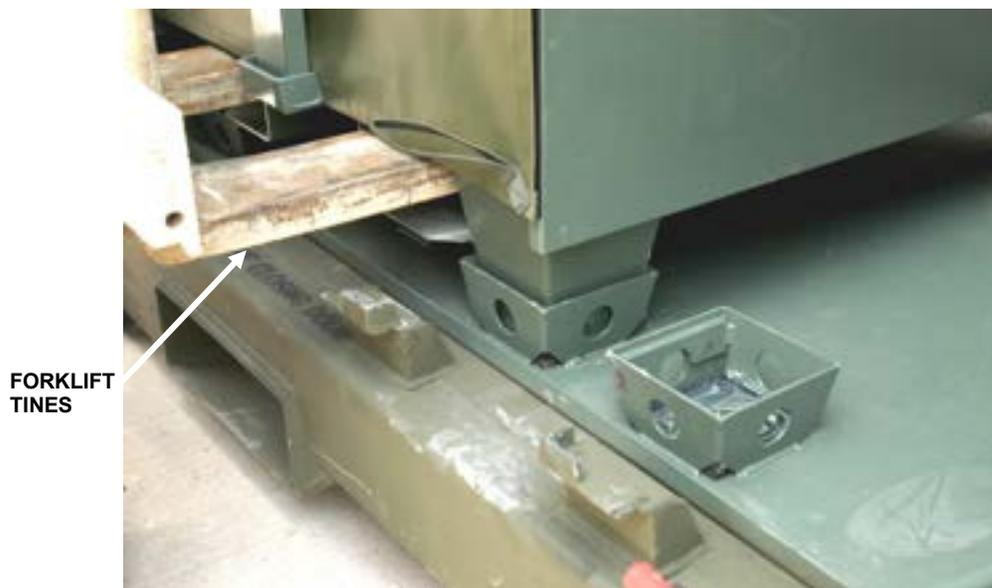
5. With the assistance of a ground guide, insert tines into module.
