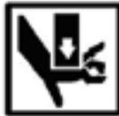
The container door release grip has limited room allocated for hand space. This creates a pinch point at the handles when closing the door. Place the door handles in the closed position after opening the doors so they will fold against each other.
