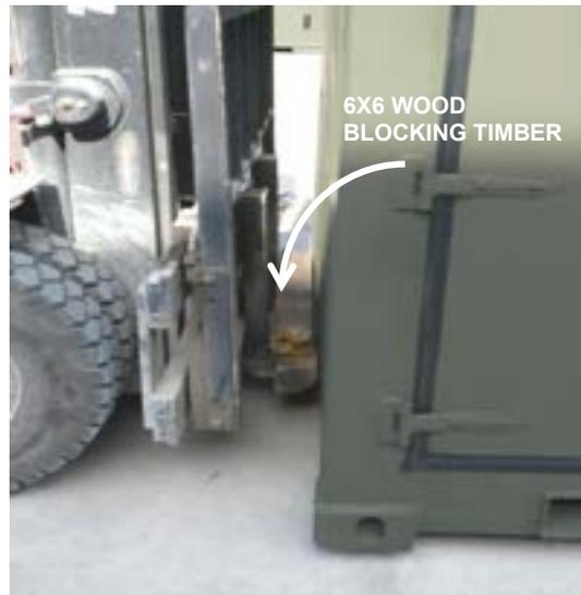
Using ground guides, restart the forklift and slowly move the FPU-8-2 forward. As the FPU-8-2 horizontal interconnectors approach the BOH-CARGO-12-1 corner blocks, maneuver the MHE to ensure the ears of the connectors are fully engaged into the openings of the corner blocks on the BOH-CARGO-12-1.
