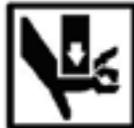
The container door release grip has limited room allocated for hand space. This creates a pinch point at the handles when closing the door. Place the door handles in the closed position after opening the doors so they will fold against each other.
