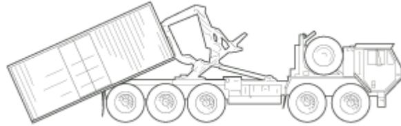
Loading and unloading via the PLS or LHS must be accomplished as indicated in PLS / LHS technical manuals. Loading and unloading onto and off of a M1076 Palletized Load-handling System Trailer (PLST) must be accomplished as indicated in the PLS trailer technical manual (TM9-2320-364-10).
