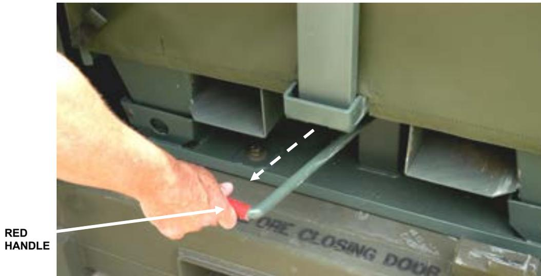
4. Adjust forklift tines to fit forklift pockets on the FPU module.
