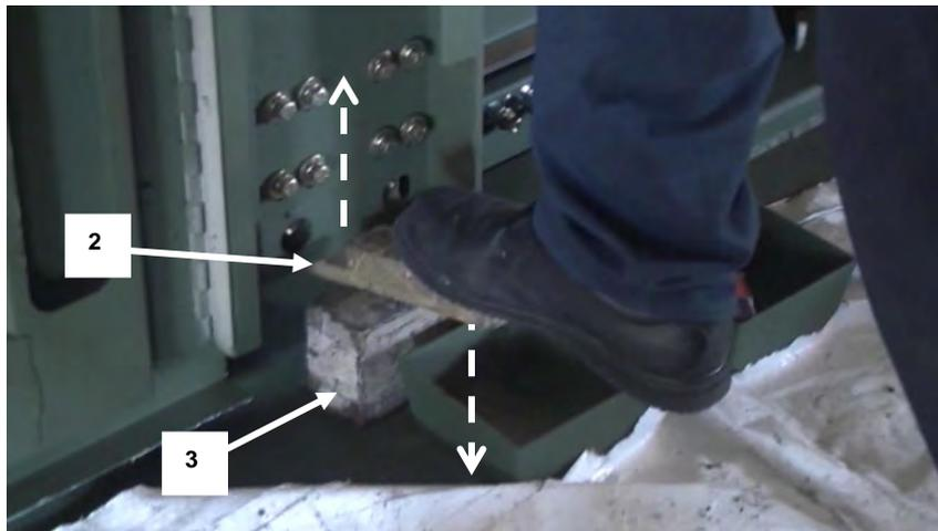
4. Release tension on the wedge and remove the wedge (2) and fulcrum block (3).
