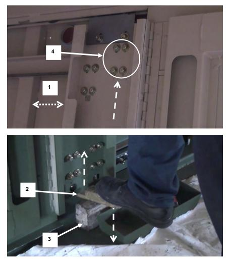
4. Release tension on the wedge and remove the wedge (2) and fulcrum block (3).
