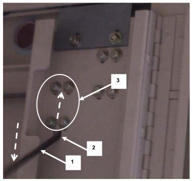
5. Obtain a large screwdriver (1) to adjust the position of the lower top bearing.
