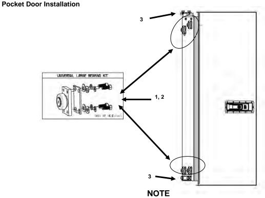
Do not install the small bearings (3) top and bottom at this time.
