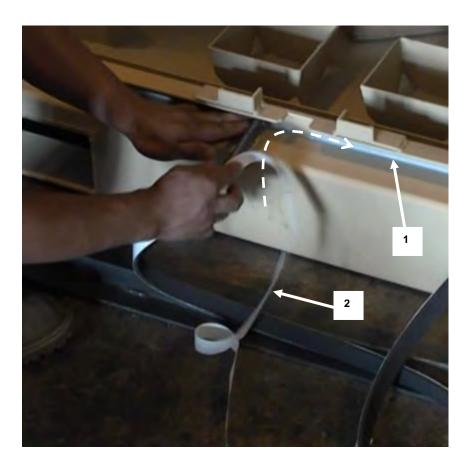
1. The lower frame seal is applied to the back edge (1) in the same fashion as the upper frame seal. 2. Peel off the paper backing (2) as you go, apply the seal and trim at the end of the run.
