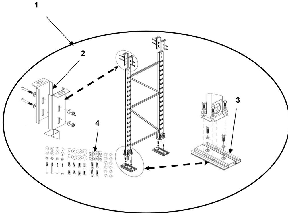
FIGURE 44 VERTICAL RACK FRAME
