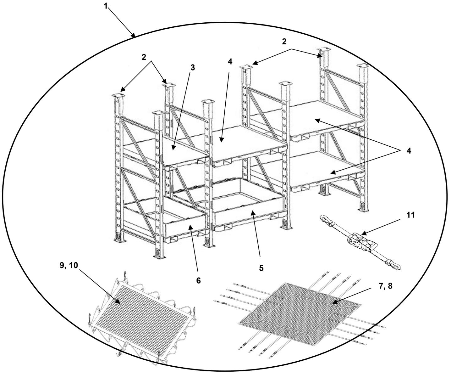
FIGURE 47 BULK STORAGE AIDS 12 FT COMPARTMENT
