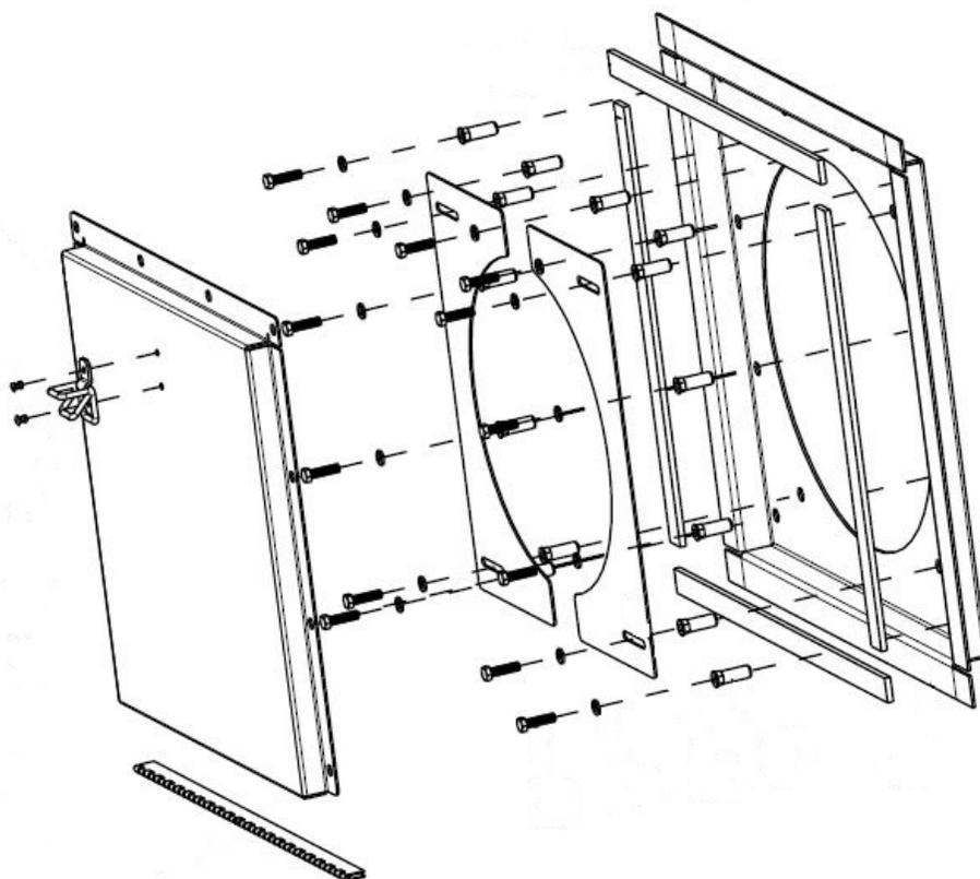
FIGURE 53 ENVIRONMENTAL CONTROL UNIT (ECU) OPTION
