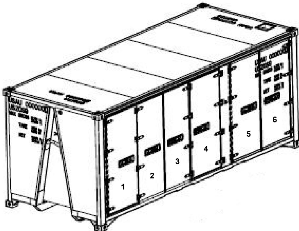
FIGURE 32 FPU-20-3 DOOR ASSEMBLIES #1 THROUGH #6
