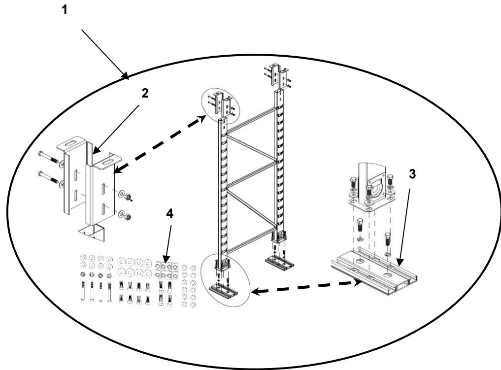
**FIGURE 18 VERTICAL RACK FRAME**
