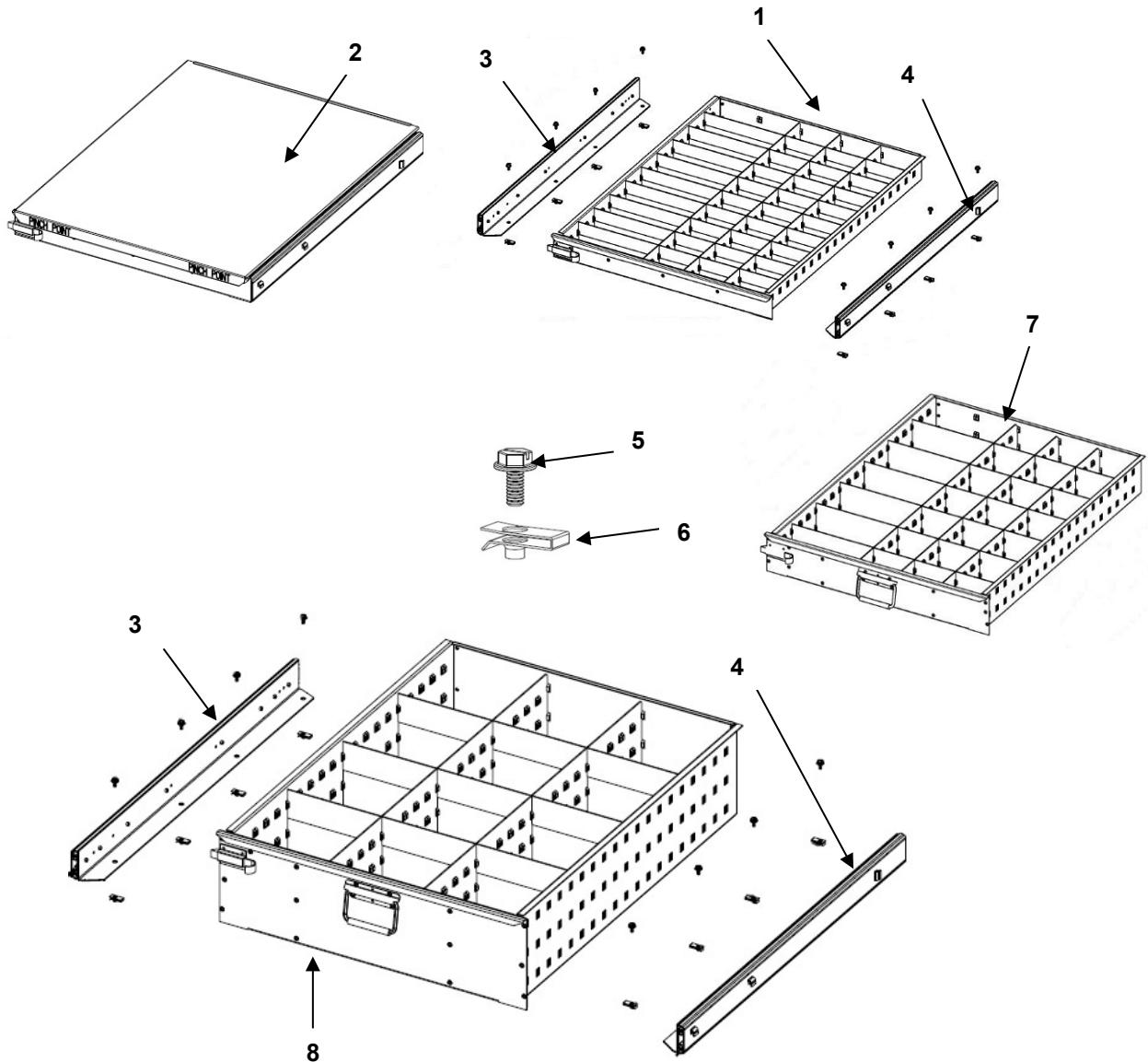
**FIGURE 33 STANDARD MODULE DRAWERS 4" THRU 8"**
