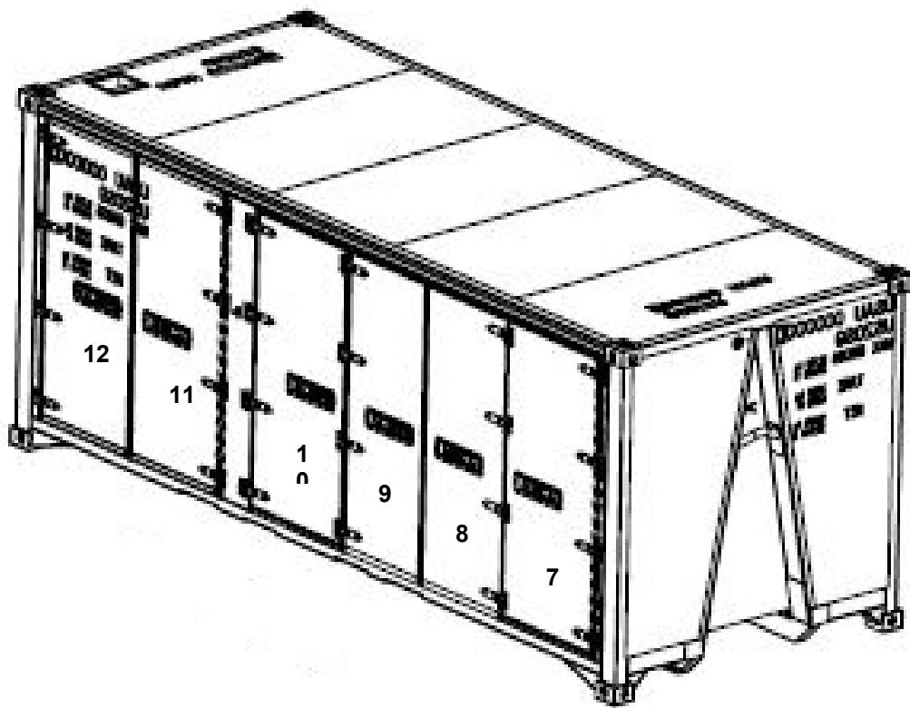
**FIGURE 7B FPU-20-3 DOOR ASSEMBLIES #7 THROUGH #12
