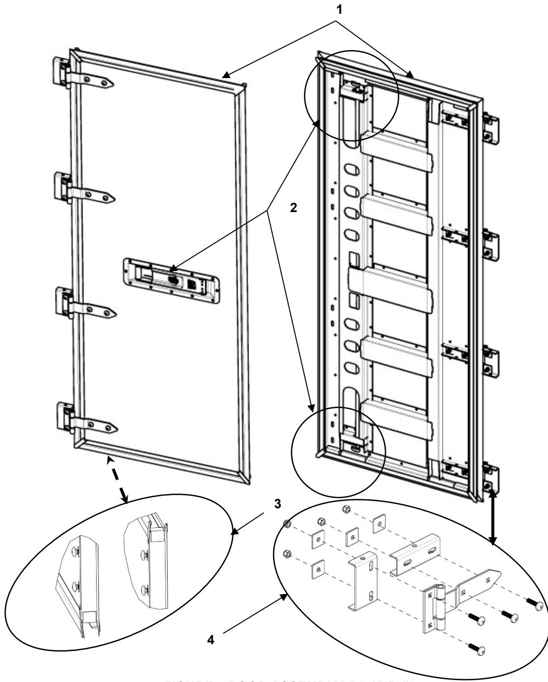
**FIGURE 9 DOOR ASSEMBLY # 2 AND #9**
