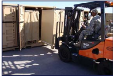
Standard FPU Module Moved by Forklift
